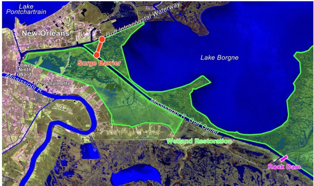
to undertake a comprehensive study of MRGO. Their study should consider how existing projects—such as the rock dam at Bayou la Loutre and the surge barrier near the Gulf Intracoastal Waterway—can be combined effectively with wetland restoration. The combination of hurricane protection structures and restored wetlands will reduce storm surge and protect communities such as the Lower Ninth Ward, New Orleans East, and Chalmette.
