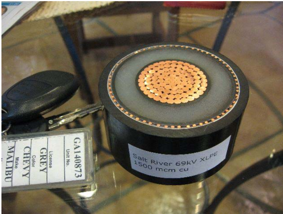
Section of underground 69 kV transmission line
