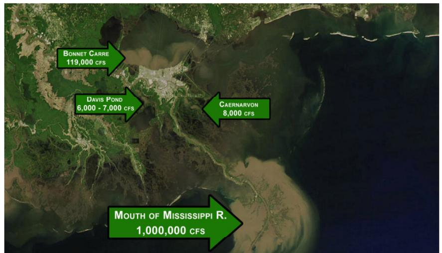
Most of the river diversions in coastal Louisiana are small and do not carry much sediment. The Davis Pond and Caernarvon freshwater diversions are illustrated above. The Bonnet Carre spillway is only opened for flood control - but also provides an unintended example of pulsed operation. Pulsed sediment diversions will help capture the **millions of tons of sediment that are lost** from the mouth of the Mississippi River to the Gulf of Mexico.
