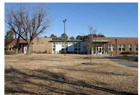
The lawn in front of the Student Services Building at Wilson Community College has regrown over the land where geothermal boreholes were drilled.
