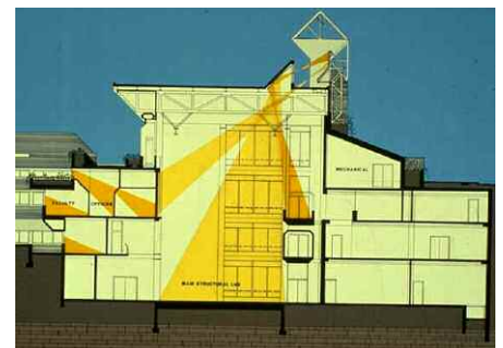
Innovative daylighting strategies channel sunlight to all levels of the University of Minnesota's Civil Engineering building.
