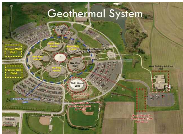
Lake Land College geothermal plans. Red lines show progress to date. Yellow lines outline future installations.
