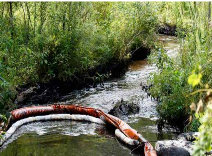
BOOM CAPTURING OIL OFF THE SURFACE OF THE KALAMAZOO RIVER AFTER THE 2010 SPILL. PHOTO CREDIT: GREENPEACE USA
