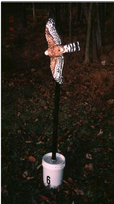
Sharp-shinned Hawk silhouette attached to a post and placed in cement for stability.
